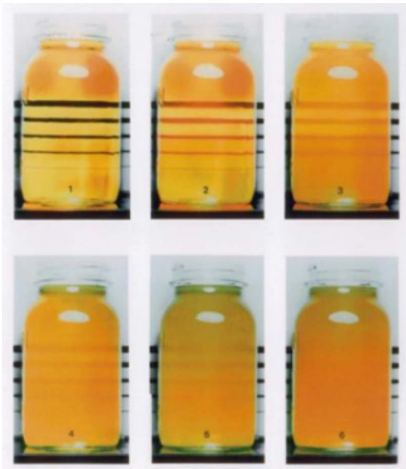
FIGURE 48B: ASTM D4176 STANDARD VISUALLY MEASURING HAZE
